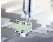
process has been tested and passed lead integrity per MIL-STD-883 M2004 condition B2 and Adhesion of Lead Finish per MIL-STD-883 M2025. In contrast to 3<sup>rd</sup> party lead attach facilities, MtronPTI is also able to perform 100% pre and post lead-attach electrical parameter and gross/fine leak testing on products.
